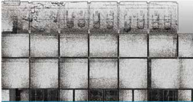
Rotating scanning making the top and bottom data uniform and the corner data complete
